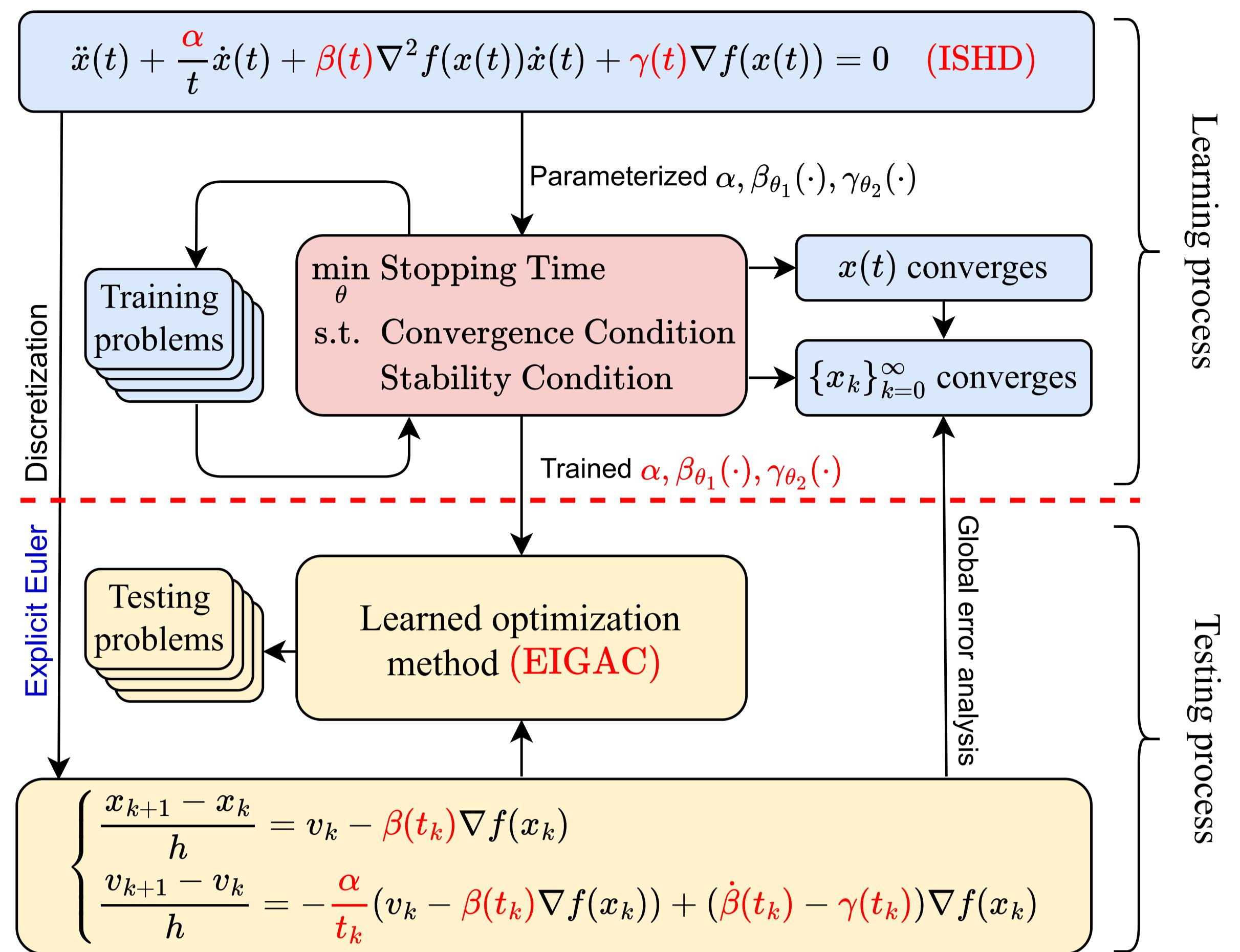
**L2O Framework:** minimize the expectation of stopping time under conditions of convergence and stable discretization
